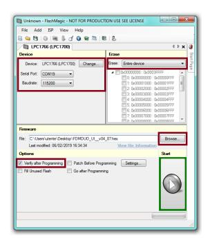
Check the communication with the FDM-DUO clicking on "ISP" and then on "Read Signature". If the communication with the FDM-DUO is working, a new window with some device information is opened.
