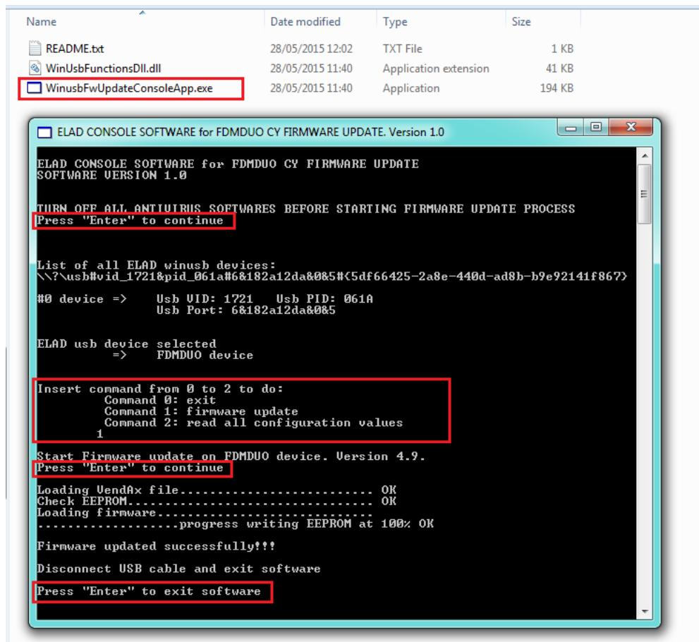
**Do not disconnect the USB cable and do not turn off the FDM-DUO.**
